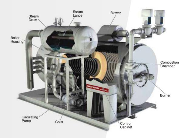
**BOILER TYPE:** Multiple parallel coil, watertube type, forced circulation, forced draft fired.
